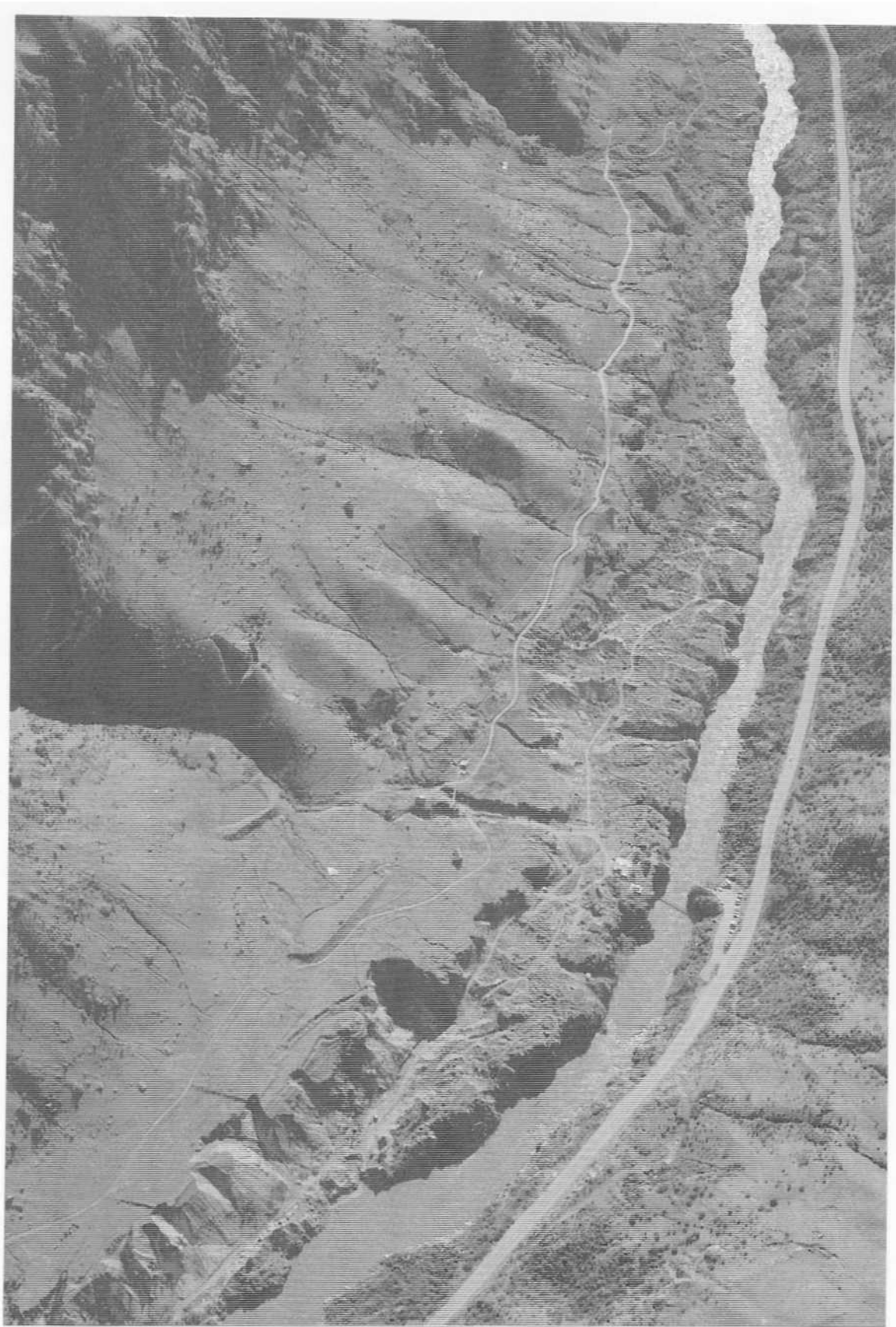
Figure 25 Oblique aerial photograph of Kawarau Goldmining Centre. Note steep bluffs above site, the storage dams below the prominent gully at left, head races entering the sluiced areas, and tail races cut through the Queen's Chain (centre). The interpretation track is prominent.
