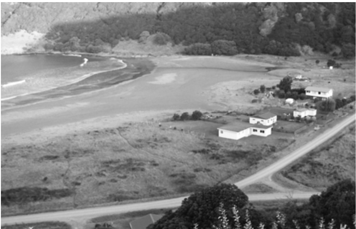
Plate 11 Site 67, Onepoto, Horseshoe Bay, East Cape, 1 April 1992, rated 33. This accreting (0.5 m/yr) sandy beach has a very lowland elevation and gradient, and experiences high storm wave run-up levels which frequently extend inland through the houses to the road paralleling the beach.
