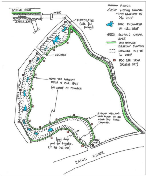
Figure 28. An example of a design to restore a degraded oxbow bend, with sloping of banks to improve access for matuku-hūrepo, and increased length of wetland vegetation. Kaihū River, Northland. *Source: Burns 2015.*
