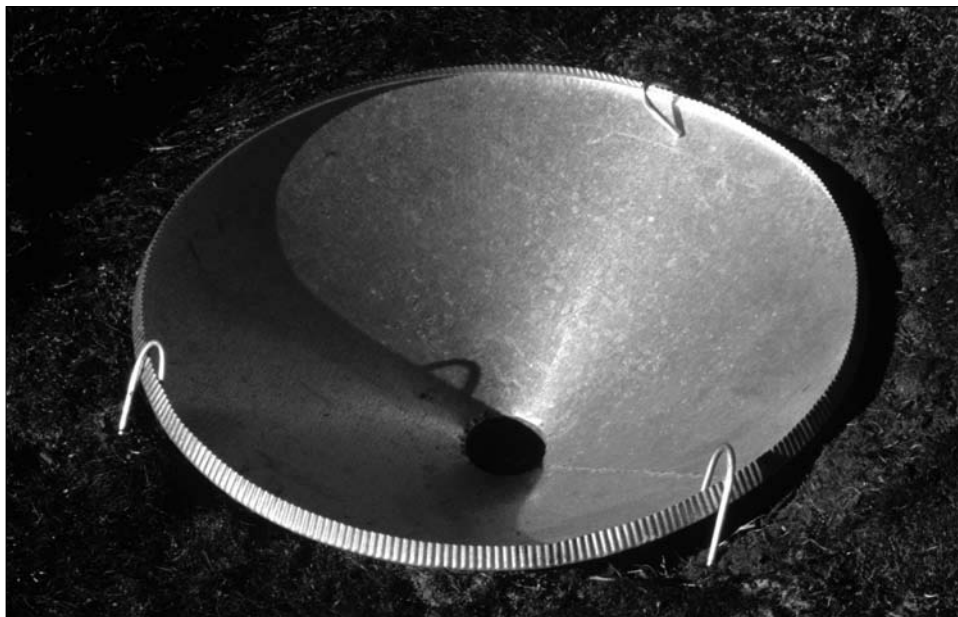
Figure 4. Galvanised iron tray used to sample ash deposited by the fires.
