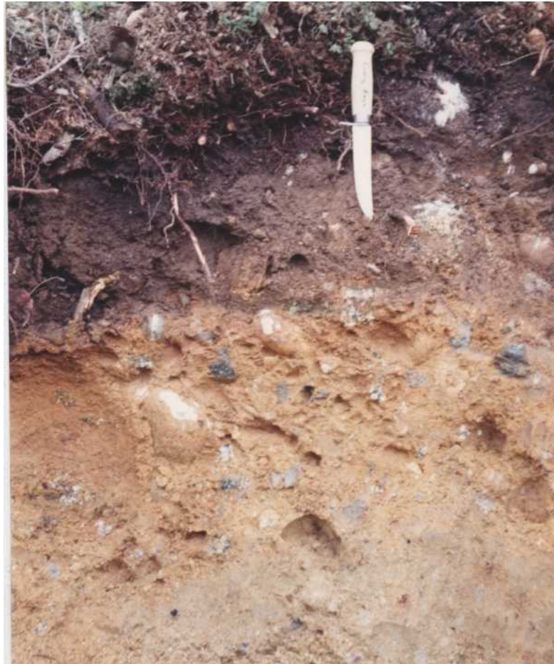
FIGURE 3. PROFILE OF AHAURA SILT LOAM. THE KNIFE IS 23 CM LONG.
