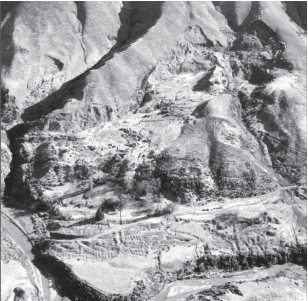
Figure 14. An oblique aerial view (looking southwest) of the southern end of Macetown. High on the hillside is a hydraulic sluicing scar (J on Map 1, pp. 10-11), with the tailrace leading off to the left cut through earlier ground sluicing tailings (K on Map 1). The 'tracks' that appear to follow hillside contours are the remains of supply and head races. Below, several building sites and Macetown's surviving timber building (H on Map 1) are located in the trees, with the regular patterns of hand-stacked ground sluicing tailings on the flat in the foreground (K on Map 1). Photo: K. Jones, Department of Conservation, Wellington.
