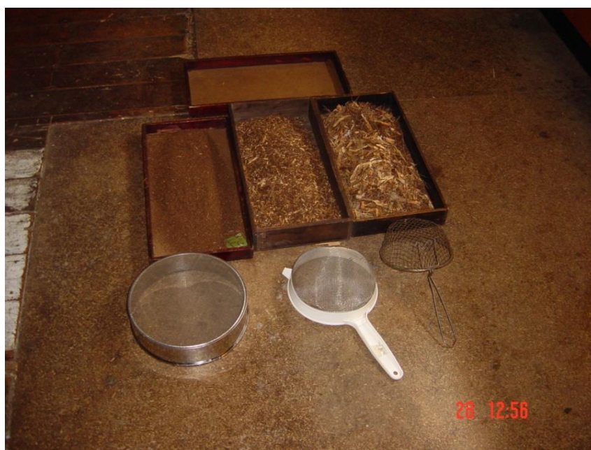
Figure 3. Use three sieve mesh sizes to sort coarse to fine material.
