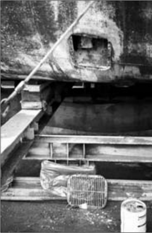
Figure 7. Seachest intake and grill.
