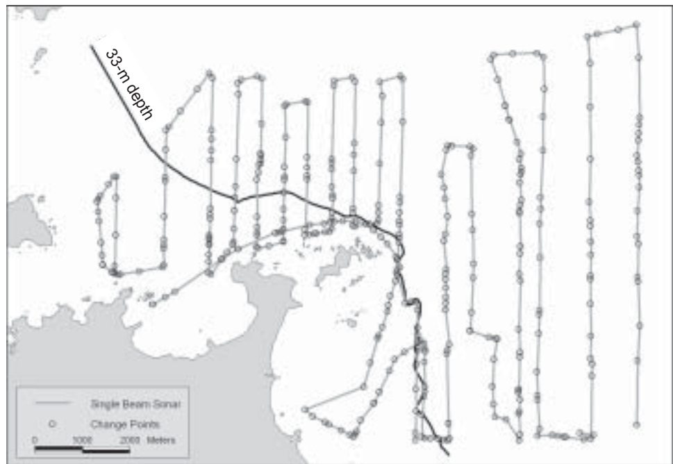
Figure 3. Single-beam sonar survey tracks. 'Change points' are positions on the sonar tracks where the habitat classification was recorded as changed from one type to another. Note: Some change points were marked only to denote change in track direction.
