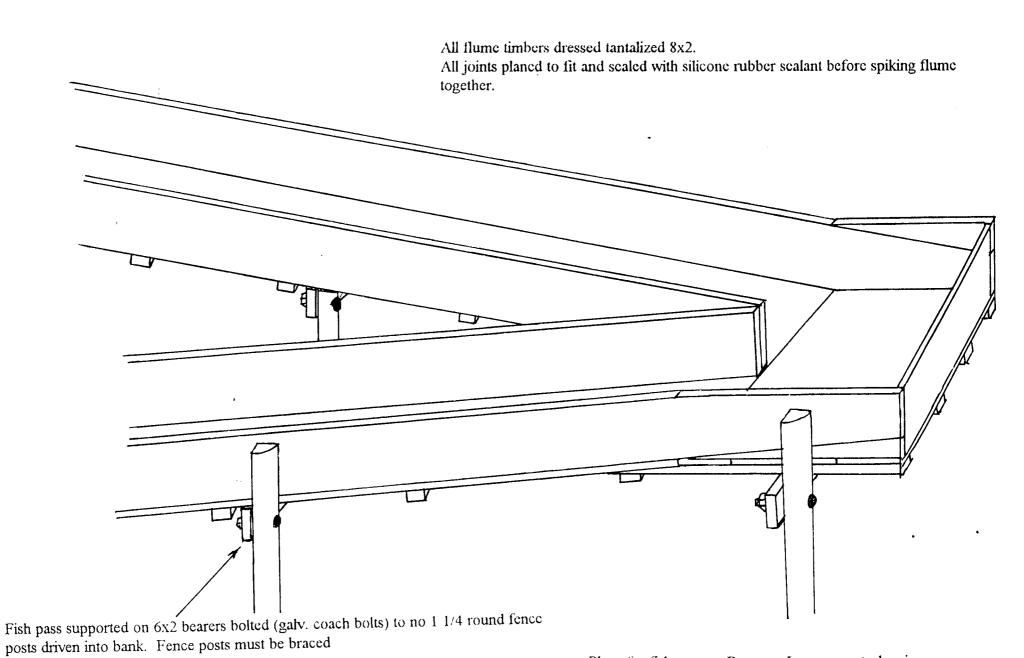
Plans for fish pass on Braemar Lagoon control weir Sheet 3 DETAIL OF TURNING POINT OF FISH PASS Butyl rubber flap nailed to flume with galv. flathead clouts Flap is weighted and dropped into water above flume to seal fish pass entrance
