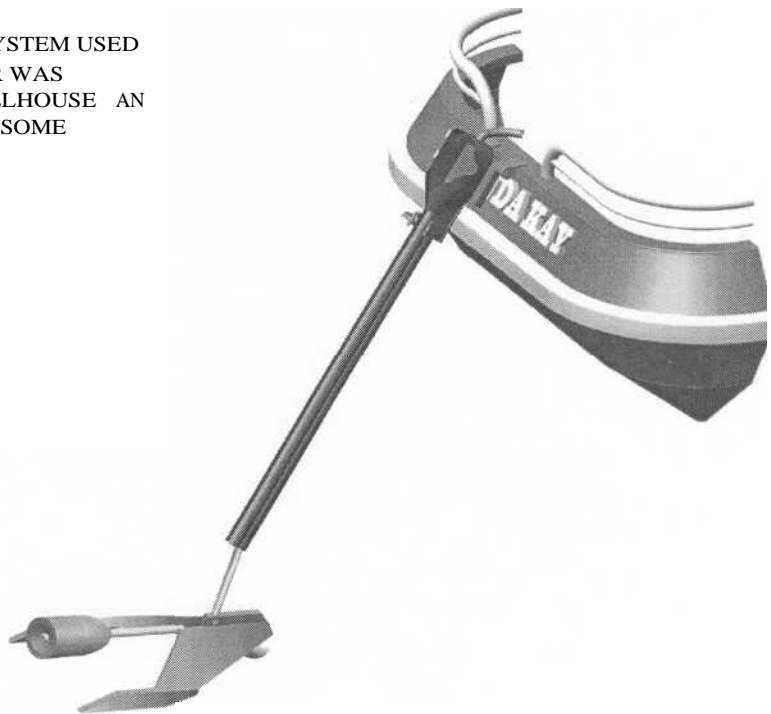
FIGURE 8. CHUTE IN USE ON F.V. BRENDA KAY . THE HANDRAIL HAD TO BE RECESSED TO ALLOW FOR IT.
