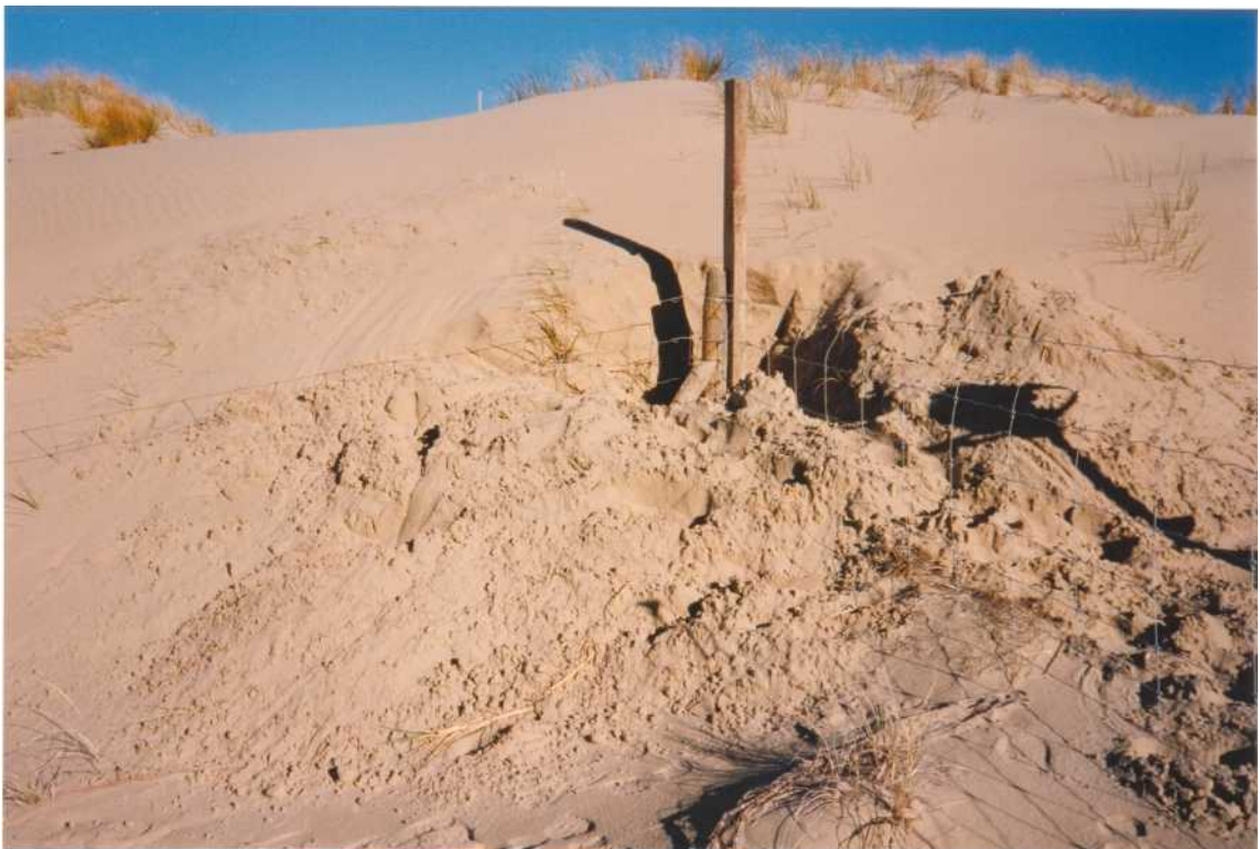
Figure 35 Sand dynamics at Plot 1. Top: NE corner of big enclosure undermined by about 30cm of sand deflation, caused by a single storm. Bottom: raising the SW corner post of the big enclosure in June 1990, just one year after construction, because of sand build-up. By mid 1997 the sand depth had increased by over 4m in this corner.
