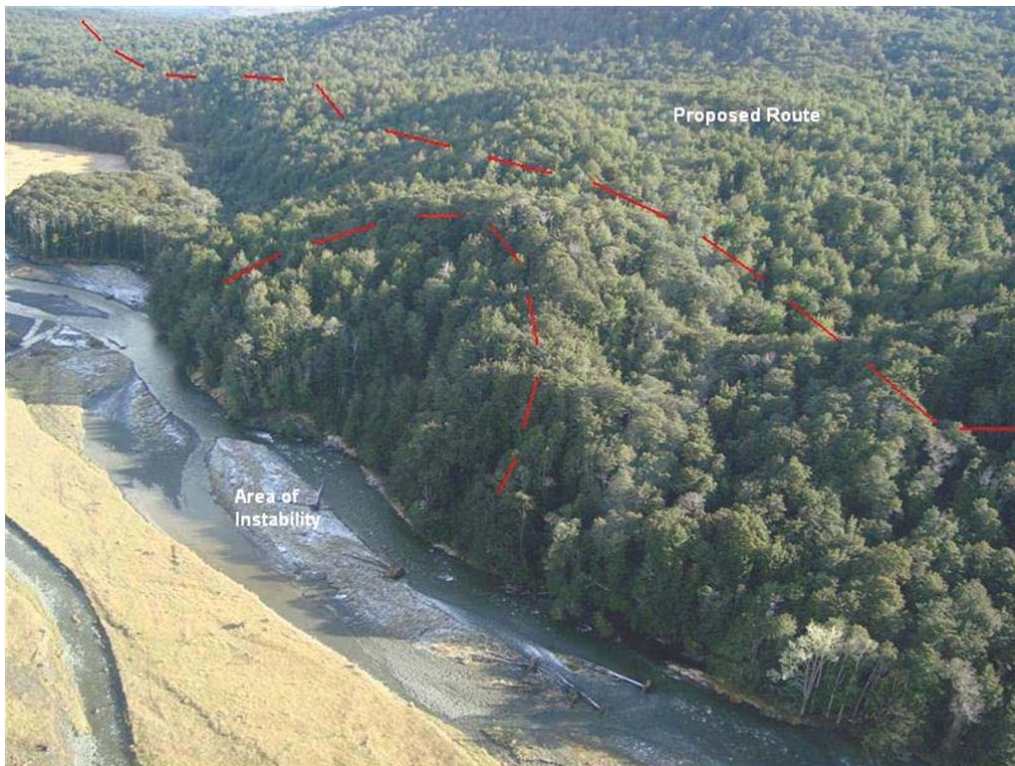
Figure 2.13 Area of instability at “Bluff Slip” on the true right of the Upukerora River at 25.5km (just downstream of Dunton Swamp).
