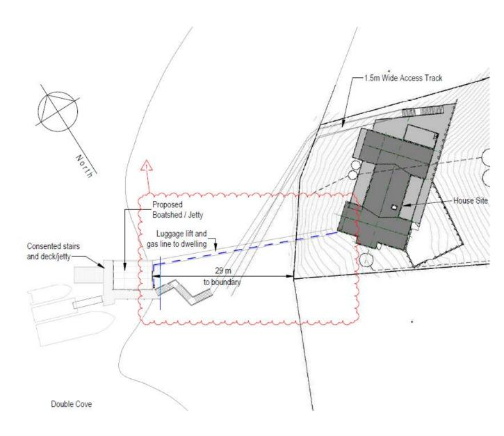
As you can see in the diagram above the two sections of the luggage trolley will run approximately 29 metres over the SFR. It is approximately 1m in width. NB: There will be no gas lines run as previously thought, these have been removed from plans.
