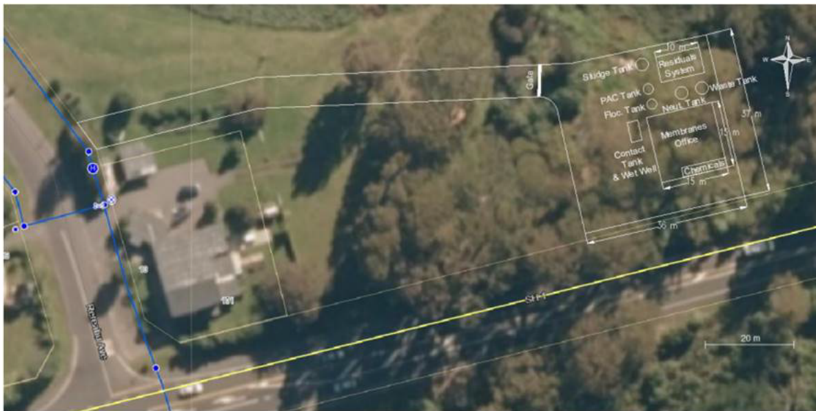
Figure 4.1 – Preliminary Hatepe Water Treatment Plant Concept Layout
