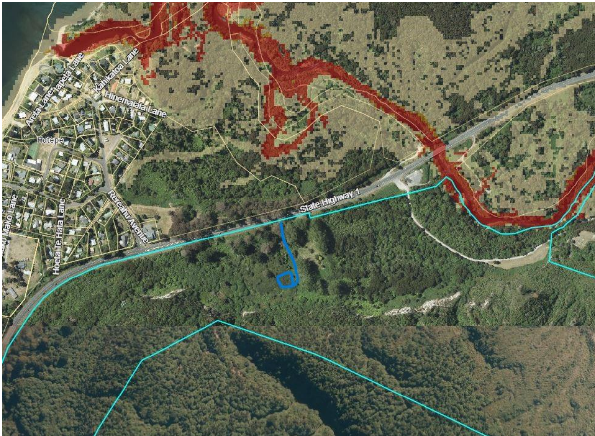
Figure 4.6. A screenshot of the TDC District Plan Flood Hazard data for Hatepe, with the proposed location of the WTP marked in dark blue, showing that the site is outside of the identified flood hazard zones.
