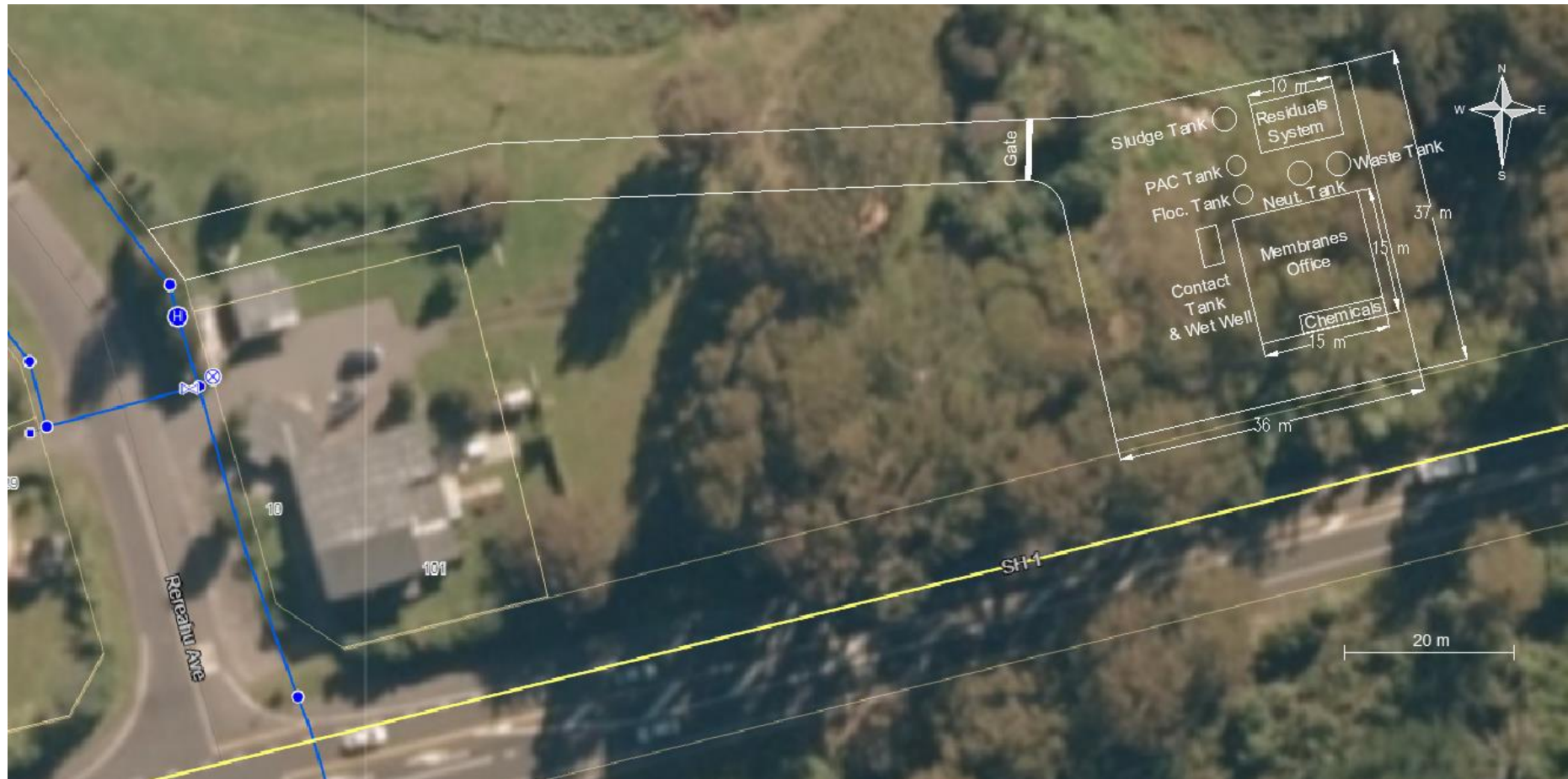
Figure 4.1 – Preliminary Hatepe Water Treatment Plant Concept Layout
