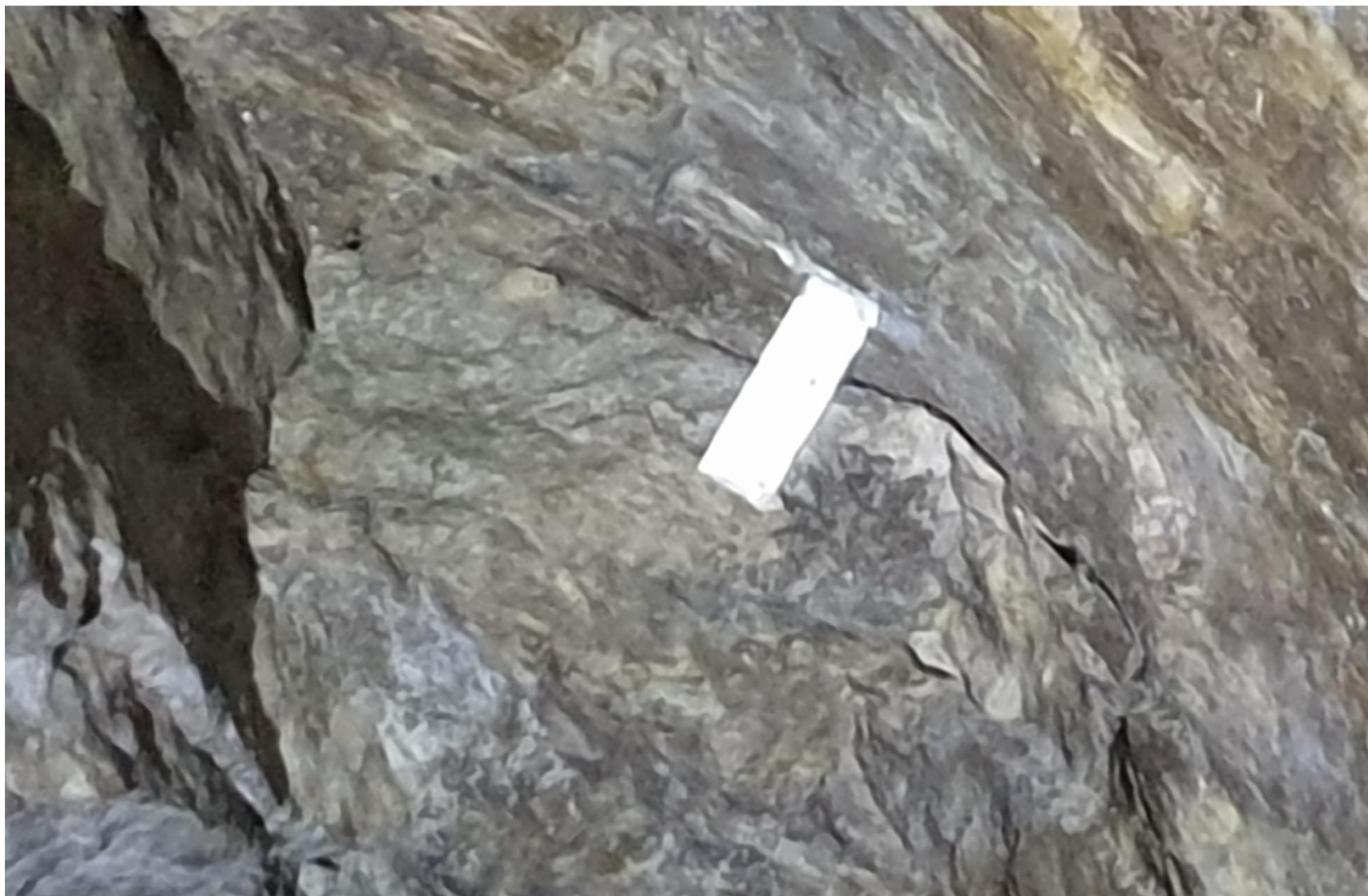
Figure 67. Photo of glass slides - to detect rock movement
