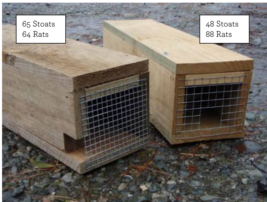
Figure 4- Side entrance tunnel (left) and mesh end entrance tunnel design (right), with capture totals at September 2011.
