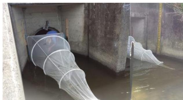
Figure 2. Large Southland sock nets were placed at the upstream end of culverts to capture any fish moving upstream (2012. Photo: Kelly Hughes)
