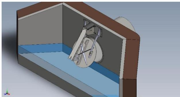
**Figure 4. Fish friendly gate (FFG) attachment showing how it delays closing and stays open when the water rises**
