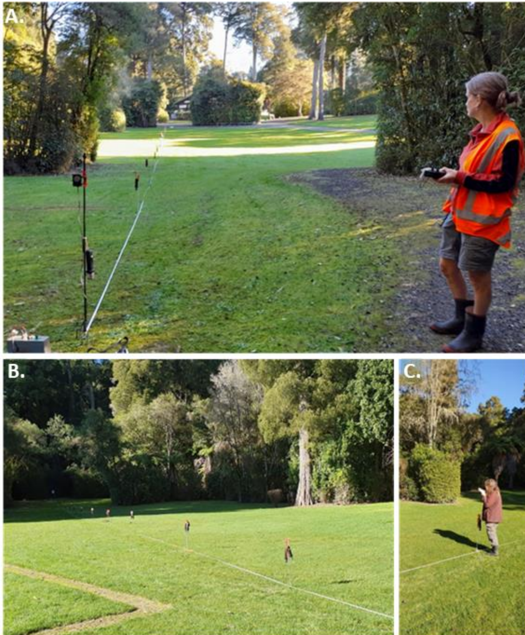
Figure 3. A. MP overseeing the lure operation beside the speaker during the pilot. The line of stakes at 5 m intervals extends 80 m directly in front of the speaker. B. Paired AR4 acoustic recorders attached to each stake C. GD manually assessing the detection distance of a hand-held detector, DOC campground, Pelorus Bridge Scenic Reserve, Marlborough, Aug. 2021.
