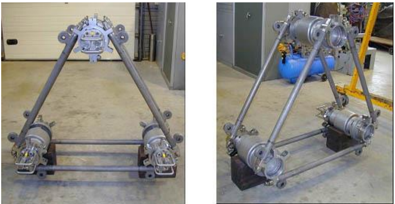
Figure 3 Triple Acoustic Source Cluster Inside Standard Delta Deployment Frame
