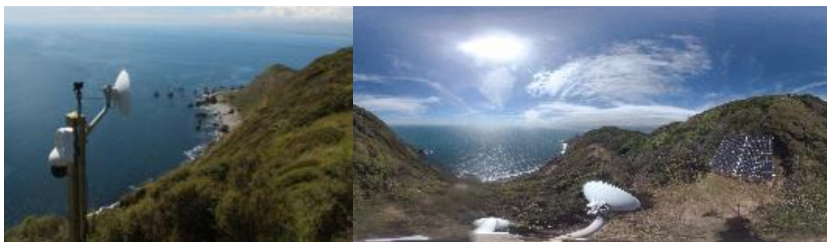
Figure 4-2: Kapiti Island fixed station telemetry site. A Garmin Virb 360° camera was integrated into the existing telemetry site at northern end of Kapiti Island overlooking the marine reserve (left) giving images (example right).
