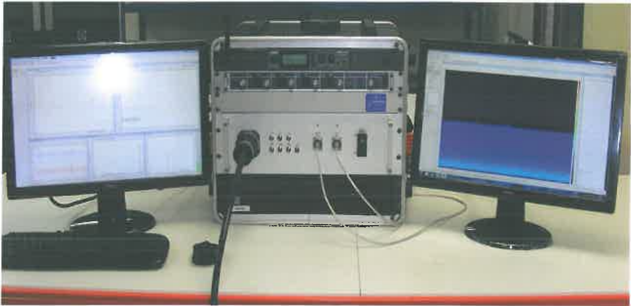
Figure 1: 8U Base unit with Rack-mounted PC and LF and HF monitors
