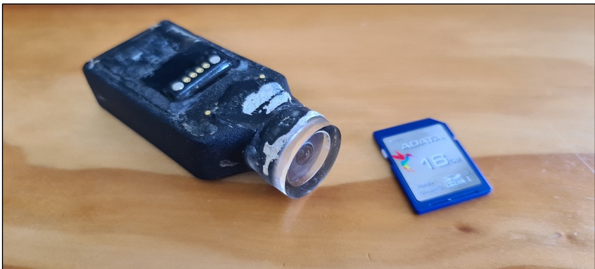
Figure 3. Eudyptes PenguCam animal-borne camera logger deployed on some hoiho during this project. SD card shown for scale.
