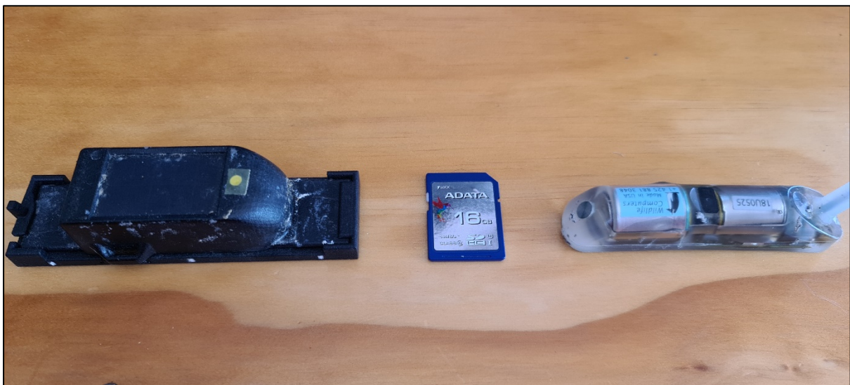
Figure 2. Transmitting devices used during four deployments in this study. Ornitela OrniTrack-25, GPS-GSM dive transmitter (left) and Wildlife Computers SPOT-275 satellite transmitter (right); SD card shown for scale. Note that the OrniTrack-25 is sitting on a magnetised base plate that keeps the unit in sleep mode; the unit is deployed without this base.
