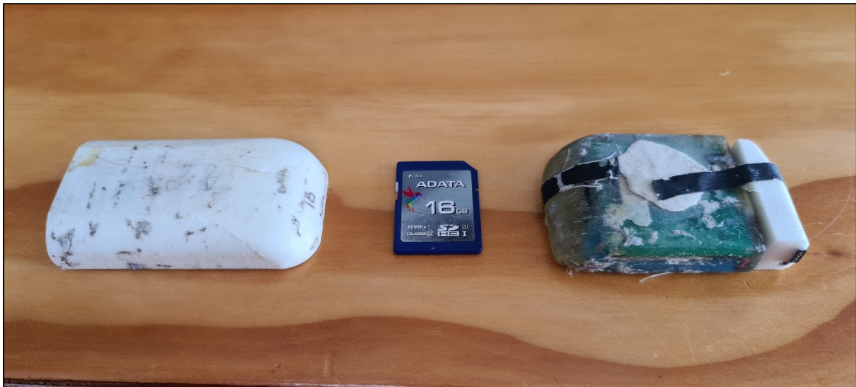
Figure 1. GPS dive loggers used in this study. AxyTrek (left) and combination of epoxy-encased i-gotU GT-600 and Axy4 TDR (right); SD card shown for scale.
