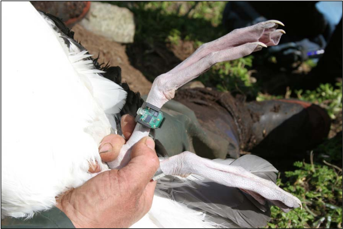
Figure 5. Light-based geolocation data logger attached to the leg of a white-capped albatross using a custom-designed leg band.
