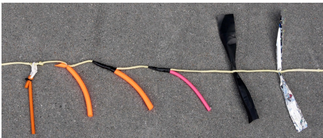
Figure 3: Tori line backbone, streamer types and streamer attachment.
