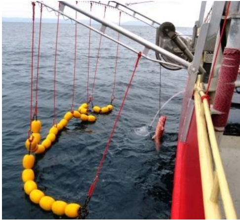
Figure 1. A bird exclusion device deployed during longline hauling. (Source: www.afma.gov.au ).
