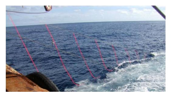
Figure 7. Streamer line with 30 m backbone, Kraton streamers at 3 m intervals, and a meshcovered 360 mm-diameter trawl float as the terminal object. The starboard trawl warp is also visible (and the port warp crosses the photo in the upper right corner).
