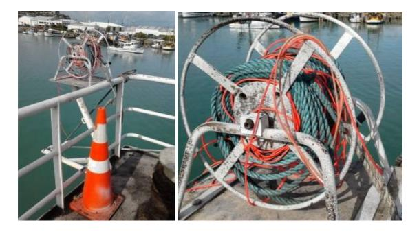
Figure 5(a, b). Storage of a streamer line on a hose reel.
