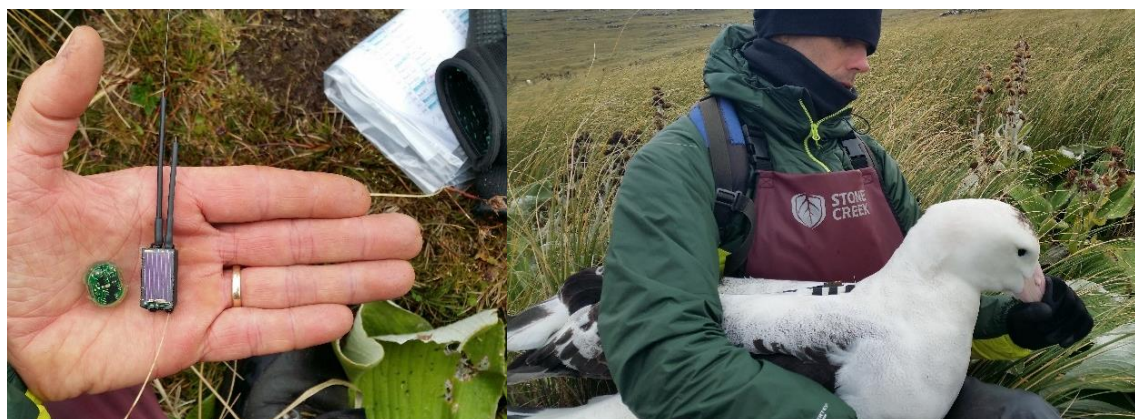
Figure 2. Left: GLS logger and solar-powered ICARUS tag. Right: Tracker fitted on Gibson’s albatross
