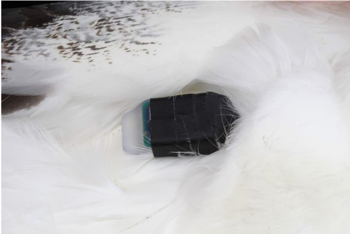
Fig. 6. An i-gotU GPS logger shortly after attaching to the back of a southern royal albatross at the Col study area, Campbell Island. Strips of Tesa tape are wrapped around tufts of feathers and the logger (Photo: P. Moore).
