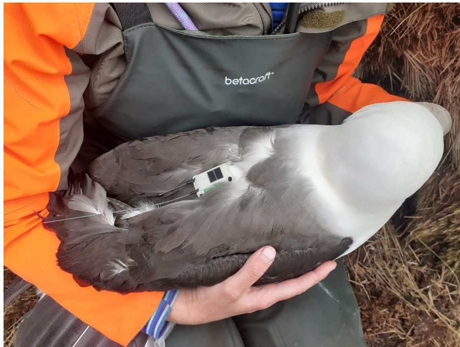
Fig. 11. Campbell albatross with a Druid PTT-GPS transmitter which has a baseplate that was attached to feathers of the back using Tesa tape, Bull Rock South, Campbell Island (Photo: P. Moore).
