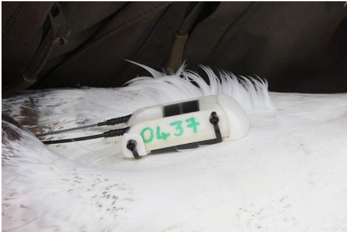
Fig. 5. A Druid PTT-GPS transmitter mounted on the back of a southern royal albatross at the Col study area, Campbell Island. A baseplate was taped to the back feathers and the transmitter was attached to the baseplate with glue and cable ties (Photo: P. Moore).
