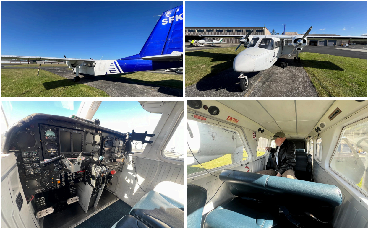
Image Set 2: Britten Norman Islander aircraft owned by Island Aviation with fixed high-wing twin engines (top left and right), pilot and co-pilot seat for data recorder (bottom left), and three rows of passenger seats for left, right, and optional belly observers (bottom right). Bubble windows may be installed on the second row, in the door and parallel window in front of the wing. Photo credits: George Shillinger/Upwell.
