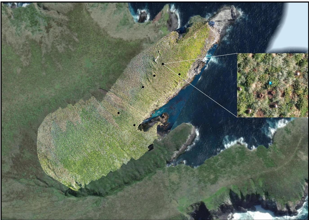
Figure 3. Ground control points on Disappointment Island (solid black circles), overlaid over an orthomosaic produced from drone photography, overlaid over adjusted aerial imagery from LINZ.
