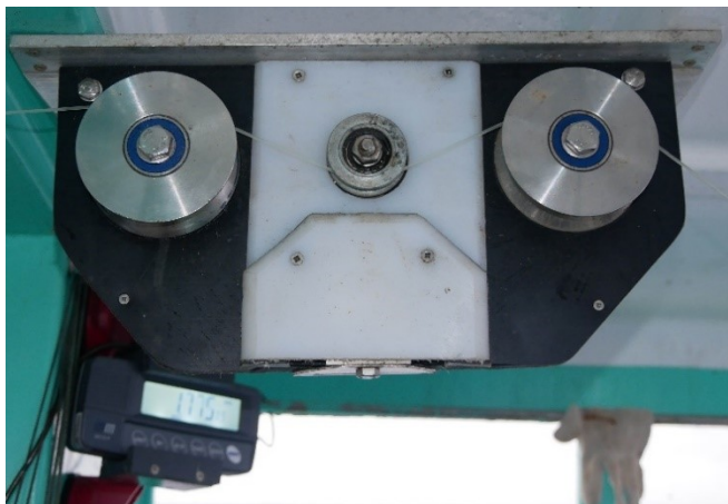
Figure 2. Photograph showing tension meter setup.
