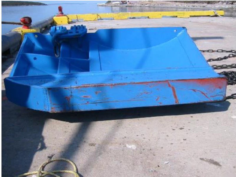
Plate A 1. Shoe of semi-pelagic trawl door indicating limited seabed contact.
