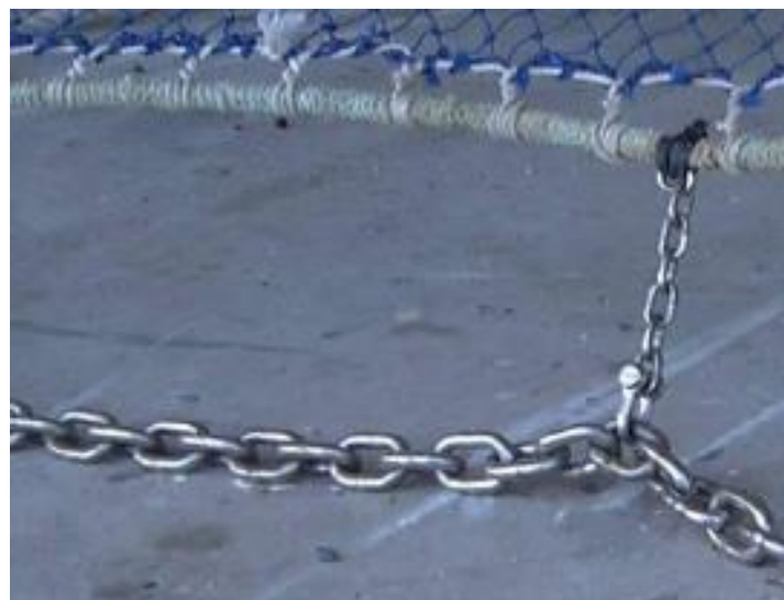
Plate 13. Typical 'Texas' drop ground chain arrangement. Source: Sterling, 2008.
