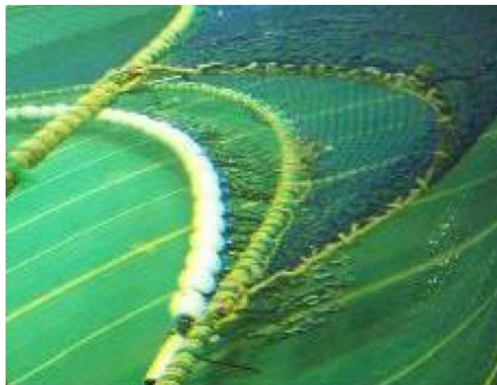
Plate 14. Soft-brush groundrope testing in a flume tank. Source: Sterling, 2008.
