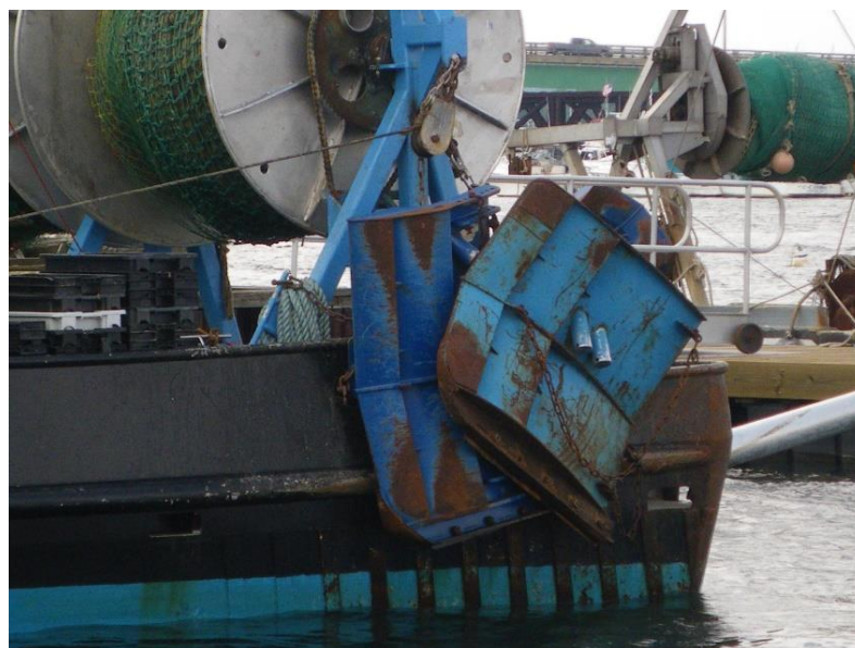
Plate A 2. The traditional trawl door (outside) and the semi-pelagic trawl door (inside). Note the difference sizes of each trawl door. Image courtesy of S. Eayrs.
