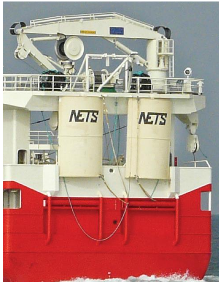
Plate 4. Lightweight trawl doors by NET Systems. Source: NET Systems (n.d.).
