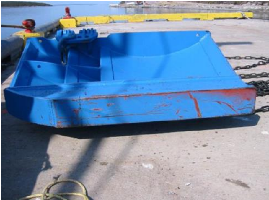
Plate 6. Shoe of a semi-pelagic trawl door indicating wear ('polish') on the bottom of the shoe. This door appears to have been heeling inward slightly, with positive tilt.
