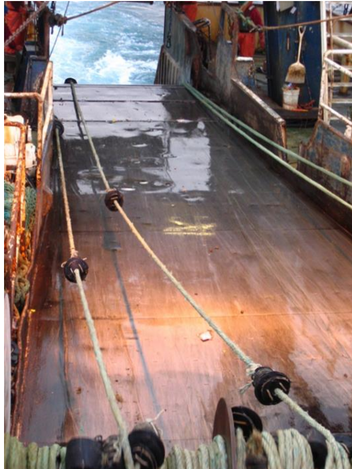
Plate 8. Cluster discs attached to trawl sweeps. Source: J. Gauvin. Alaska Seafood Cooperative.
