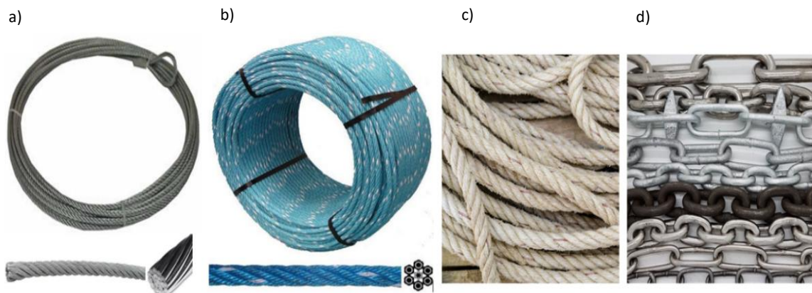
Plate 3. Common sweep and bridle materials in bottom trawling. a) Steel wire rope, b) combination rope, c) natural rope, and d) chain. Adapted from Larsen et al. , 2019.
