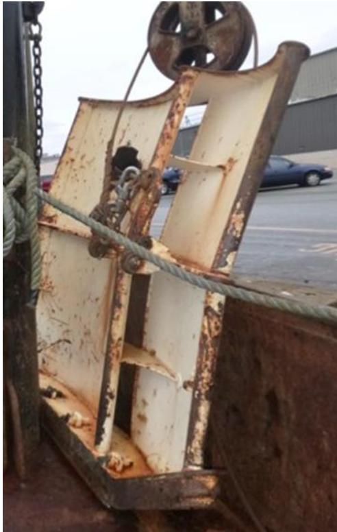
Plate A 3. The Gull wing trawl door. Image courtesy of P. He.
