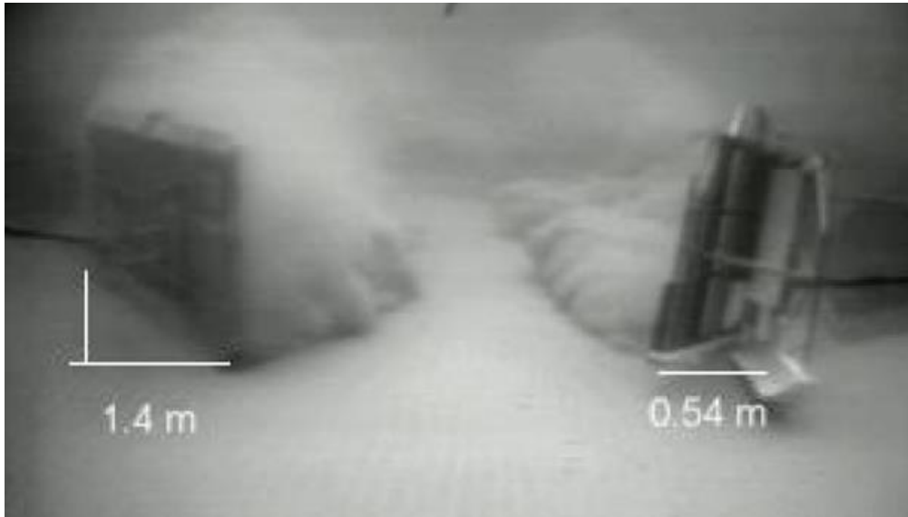
Plate 5. The effect of angle of attack on the swept width (footprint) of trawl doors. The flat rectangular trawl door on the left is operating at an angle of attack in excess of 30^\circ and the 'batwing' trawl door on the right is operating at around 20^\circ . Source: Sterling and Eayrs, 2010.
