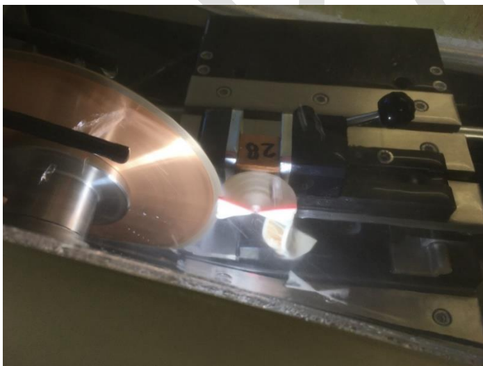
Figure 1. Cleaned vertebrae adhered to wooden stubs with epoxy resin (top panel); vertebra prior to sectioning showing laser guided sectioning transect (middle panel); classic “bowtie” sections being completed (bottom panel).
