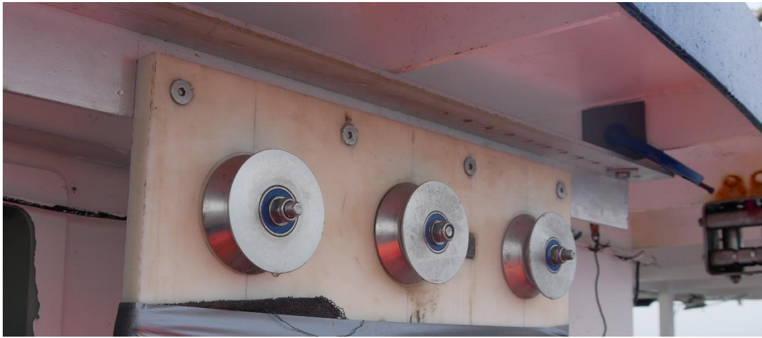
Figure 2. Photograph showing tension meter setup.
