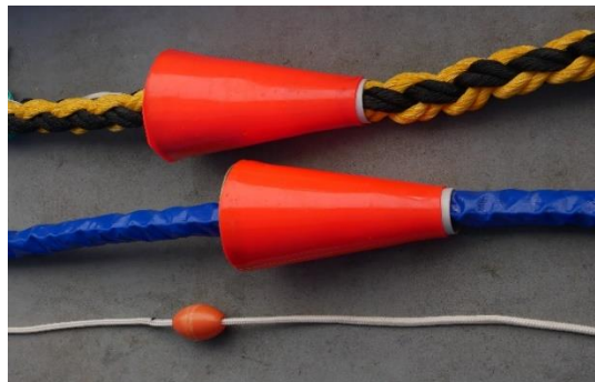
Figure 3. Photograph showing details of the tori line drag sections tested: 52 mm diameter 8 plait rope threaded through a 280 long 150 mm diameter cone, 32 mm rope covered in hose with the same cone, and 9 mm trawl braid with a gillnet float.
