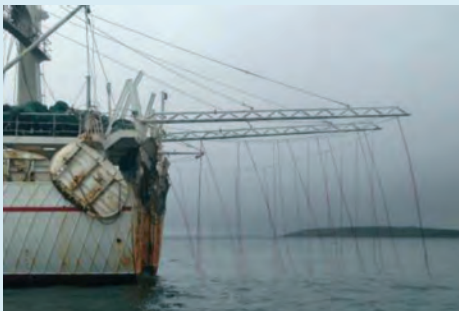
Tori line-type streamers hung from 14 m long booms on a trawler operating in the Falklands (see 'Want to know more?'). Photo: G. Parker and colleagues
