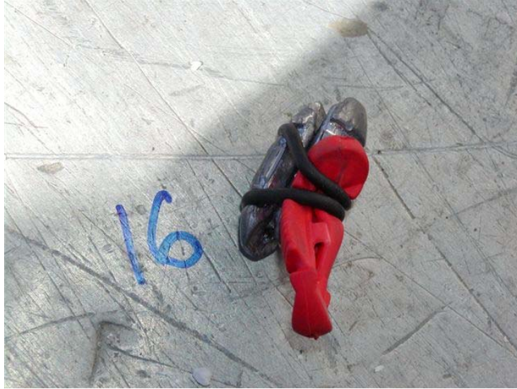
[Twisted safe lead after 100kg line break]
