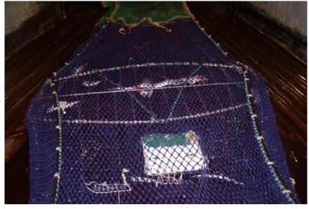
**Figure 14:** SED on deck after haul. A single frostfish (*L. caudatus*) is still retained across the bars. The placement position of the camera close to the apex of the closed escape hole and within the lengthener can be clearly seen, April, 2009
