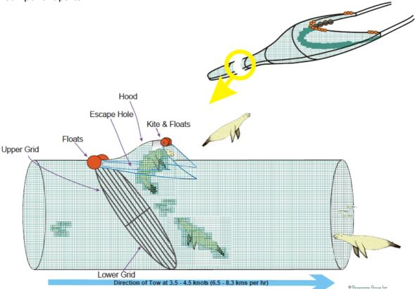
**Figure 1:** Schematic of SLED (not to scale). Note that when in operation, the codend would be attached to the net on the left of the diagram (Source DeepWater Group Ltd).
