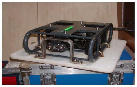
**Figure 5:** Tritech Seacorder white light camera. The Teflon base board and stainless protection bar were added to improve usability and protection. Ball point pen lying on top provides scale.
