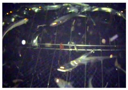
**Figure 15:** Video still of hoki impacting on grid bars during tow. Note sideways orientation of many of the hoki, second sea trial, April, 2009.
