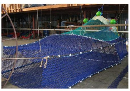
Figure 16: SED viewed from behind, final lengthener and codends attach at end closest to observer.
