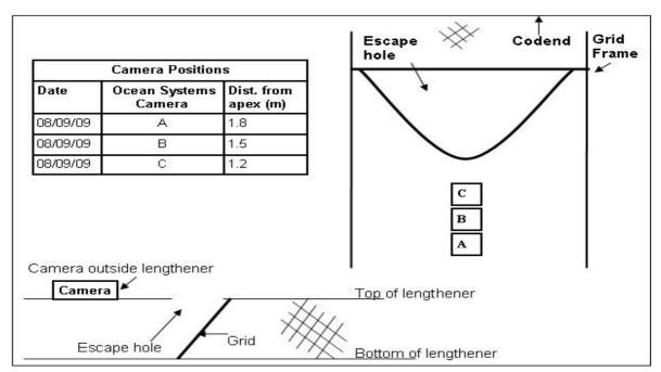
Figure 4: Camera placement for the three tows undertaken during initial sea trials, side and plan views.
