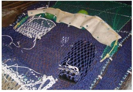
Figure 2: Both cameras fitted inside the SED lengthener, FV Taimania, April 2009
