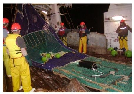
**Figure 7:** Ocean Systems camera fitted on the trawl ready for deployment. Camera light can be seen operating, *FV Taimania*, September 2008
