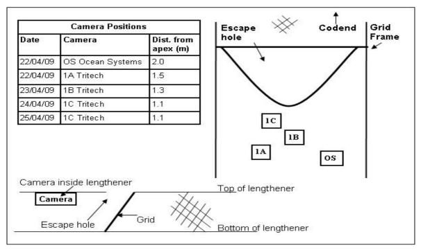
Figure 6: Camera placements for second sea trials, side and plan views. Note OS camera failed after two tows.
