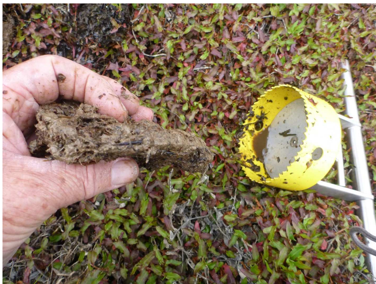
Figure 4: Hand operated corer (right-yellow) has an internal plunger to eject the soil plug from the corer. The soil plug taken (left) may include plant roots, which will be removed before analysis.
