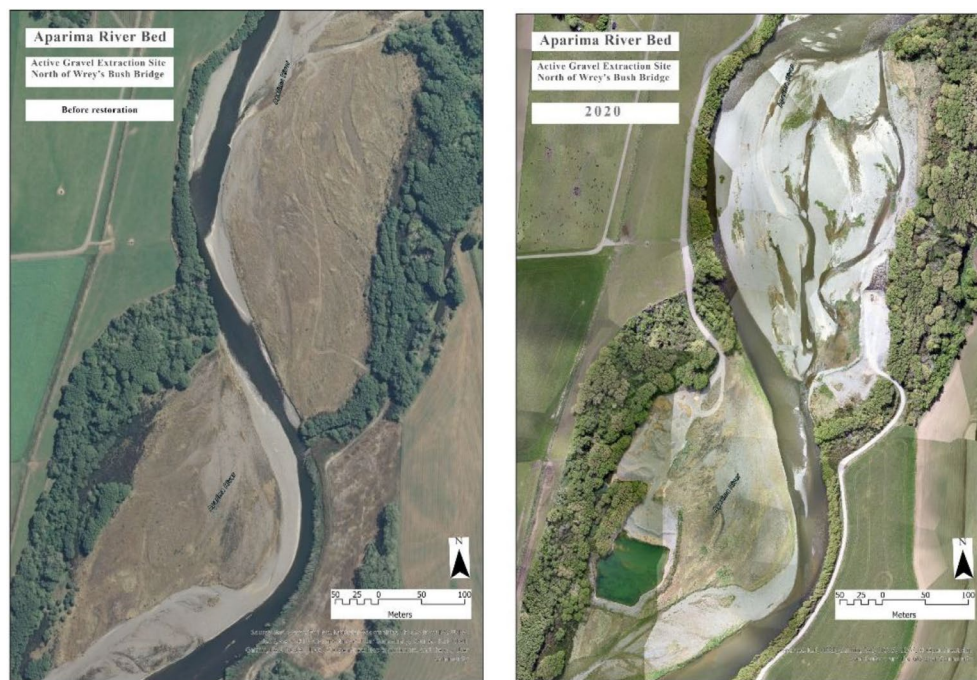
FIGURE 2 | Aerial photographs of the Aparima River. Left, 2016: Prior to application of the experimental gravel and overburden skimming technique—the river is constricted and channelized, and gravel bars are covered in exotic vegetation. Right, 2020: The experimental gravel and overburden skimming technique (RES treatment) has been applied in the top section; overburden has been removed, multiple channels and bars are visible, and conditions are intended to be more representative of the natural river, and, therefore, impact fish population health positively. The pit mining/POND treatment can be seen in the bottom left of the photo. The lower right section of the river channel is representative of the unrestored/UNRES treatment. Source: Department of Conservation. [Color figure can be viewed at wileyonlinelibrary.com ]
