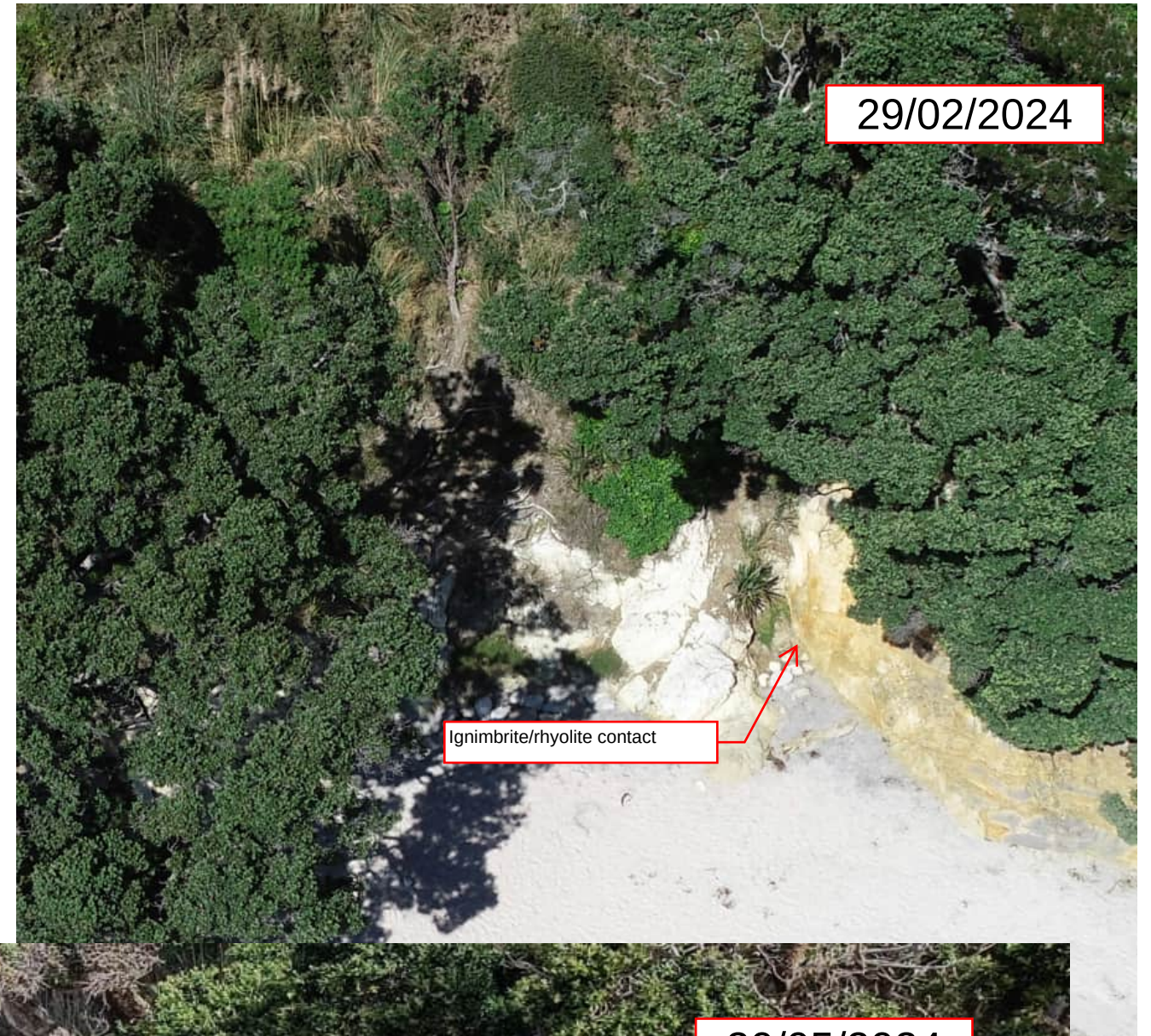
Feature 35 - Translational landslide where ignimbrite abuts rhyolite. No new movement observed.
