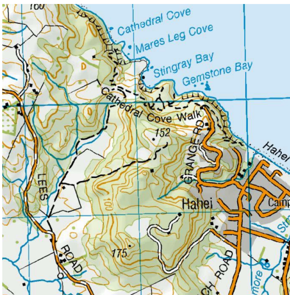
Figure 4.1: 1:50:000 Topo map (Source Topomap.co.nz / LINZ). Blue grid lines are spaced 1 km and vertical blue lines are oriented to grid north.
