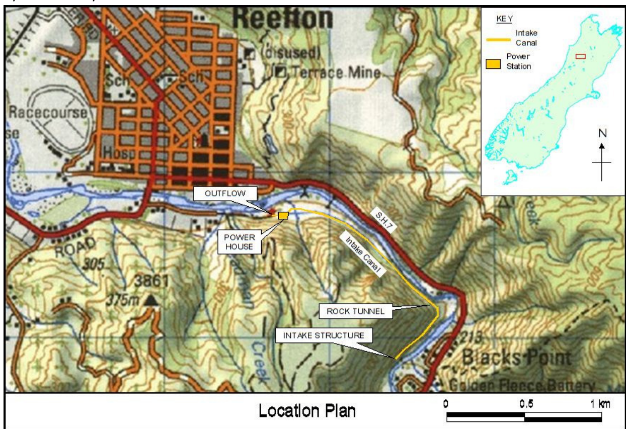
Figure 1: Location of proposed Reefton Power Scheme showing the intake location and power station site, and the 2 km of river where flows will be reduced when the power scheme is operating.
