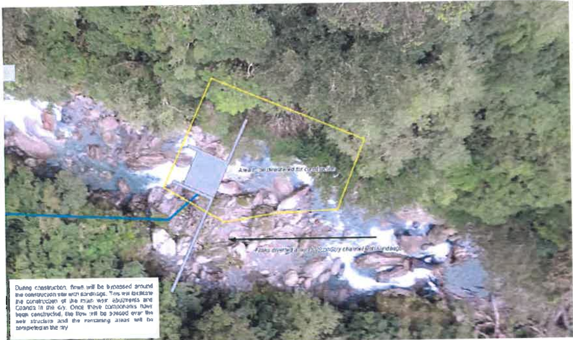
Figure 6 – Indicative plan of proposed weir and dewatering sequence
