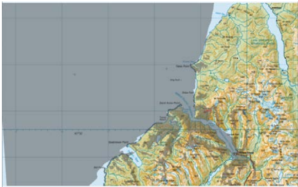
Map 2 - Radio Signal Coverage shown as the grey area, from Proposed Location (indicated in red)
